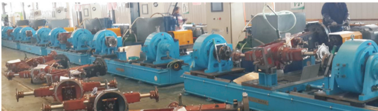
车桥测试台 (磁粉测功机) Axle test bench (magnetic powder dynamometer)
