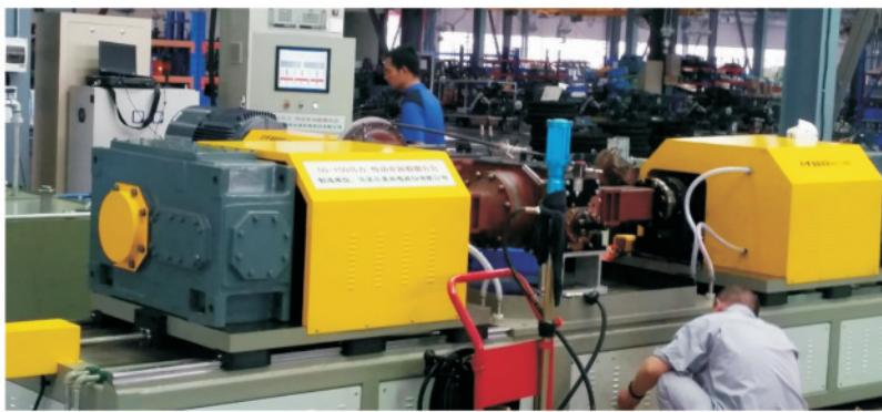
车桥测试台 (电力测功机) Axle test bench (electric dynamometer)
