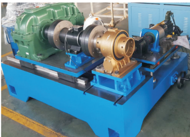
太阳能发电用减速机测试台 Reducer test bench for solar power generation
